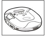
1. During stop, press PROG button until "PROG "flashes in LCD. The track number and playing order appears.
